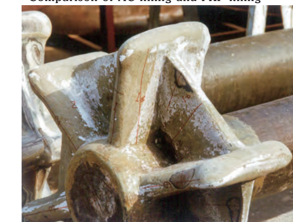
AC lining is no abrasion. (Operation terms: 12 Months)
