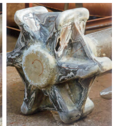
FRP lining is abrasion. (Operation terms: 6 Months)
